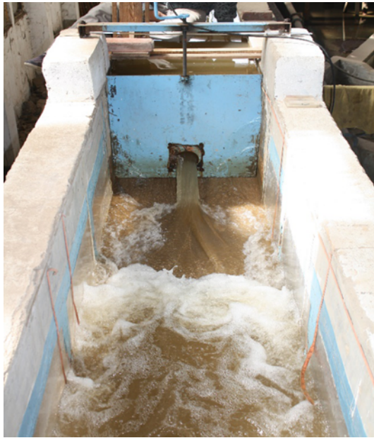
Fig. 2. Flow Downstream Sluice Gate with Orifice
